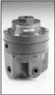
Type-600 Ratio Relay Volume Booster Uses a pneumatic signal to produce an output pressure which has high flow capacity and can be amplified.
